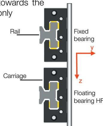
Installation variation lateral with floating bearing in the Z direction
