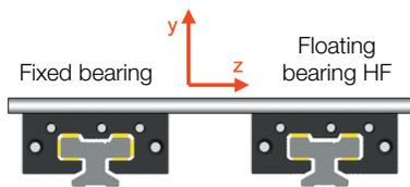
Installation variation horizontal with floating bearing in the Z direction
